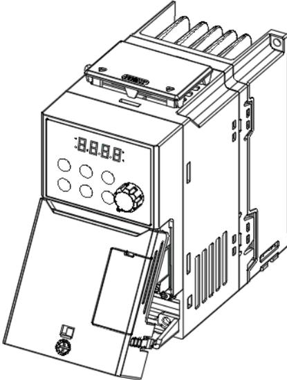
Loosen the bolt that secures the front cover (R). Push and hold the latch on the right side of the cover. Then remove the cover by lifting it from the bottom and moving it away from the front of the inverter.
