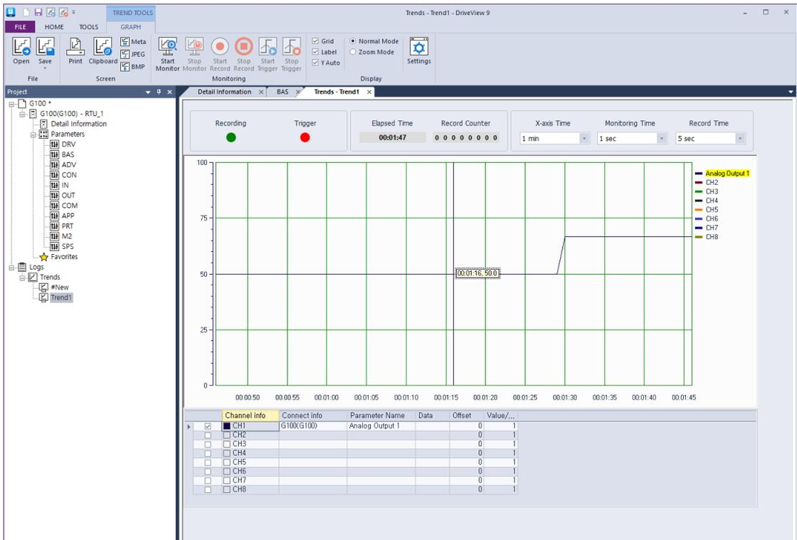
On the Trends screen of DriveView9, you can monitor the parameters in the graph form. Monitoring graphs provide 8 channels. Trends provide monitoring, recording, and trigger observation features. For more details, see DriveView9 user's manual.
