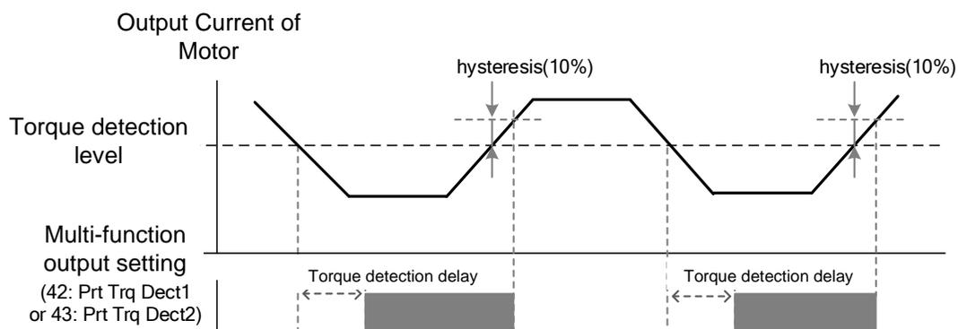
The over and under torque detection level set as OU68, 71 parameters are set as the ratio on motor's rated current.
