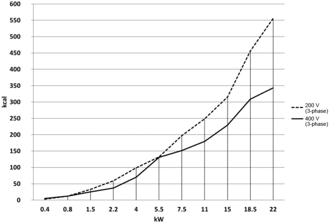
Heat emission has been measured based on the room temperature when the carrier frequency of inverter is set as default. For more information on carrier frequency, refer to **5.15 Operational Noise Settings (Change of Carrier Frequency Settings)** on page **159**.
