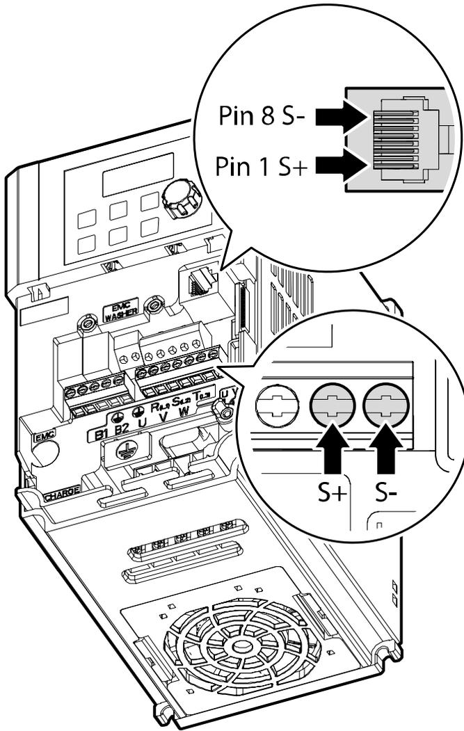
Use 2Pair STP (Shielded twisted Pair) cable (using only no.1 pin S+, no.8 pin S-/ no.1 and no.8 pins are twisted types, no.2 pin to no.7 pin are not allowed) and a RJ45 STP plug. Use a RJ45 coupler for connection between products and cable extension (Y type LAN coupler where STP can be mounted). (Use LAN standardized products for cables, plugs, and couplers: CAT5, CAT5e, CAT6.)
