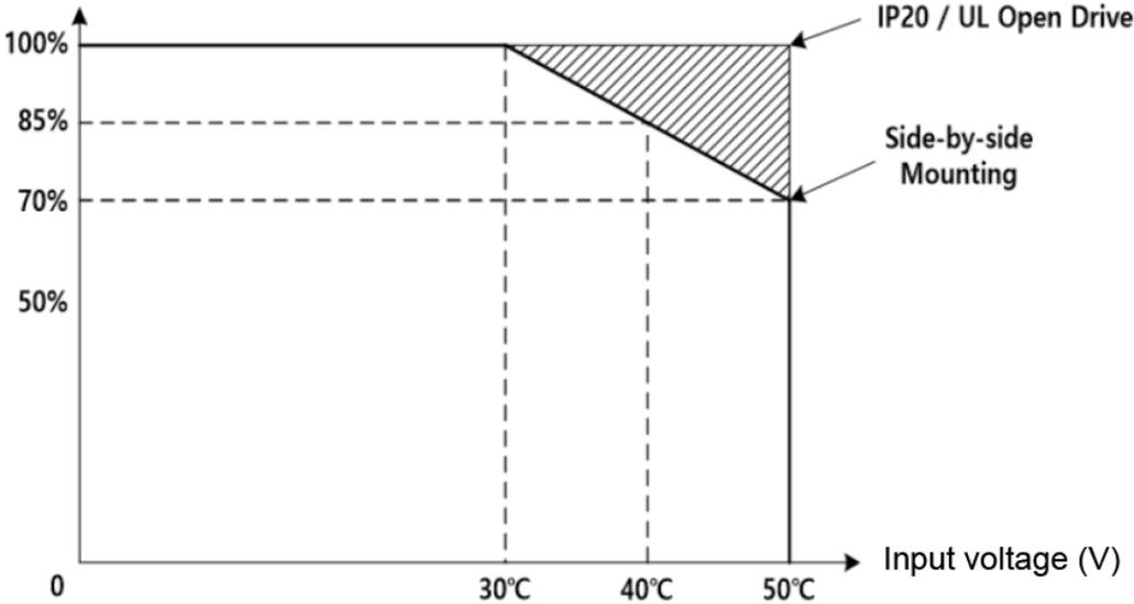
※ This graph is applied to both HD and ND. However, ND lineups include a model for 40 °C and below temperature.
