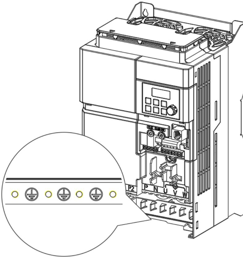
2 Connect the other ends of the ground cables to the supply earth (ground) terminal.
