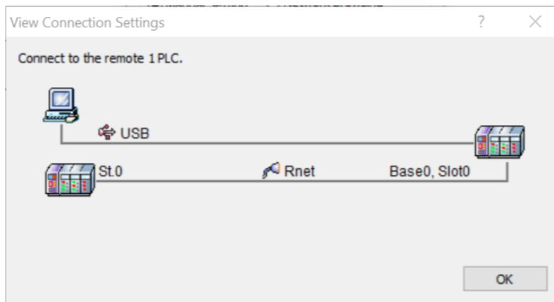
(b) Click [Setting] and set the detailed information of the RS-232C and the remote 1-stage.
