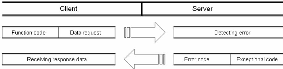
When an abnormal frame is received, the server transmits the error code and the exception code to the client. The error code is the value of the function code plus 80(Hex) value, and the exception code indicates the error details. The contents of each code are as follows.
