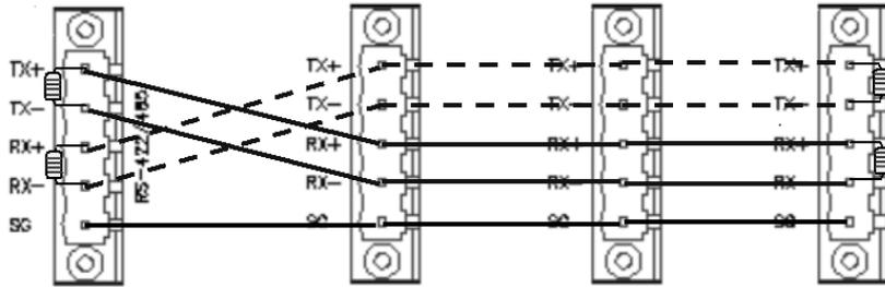
(2) How to connect the terminating resistance in case the RS-485 is connected
