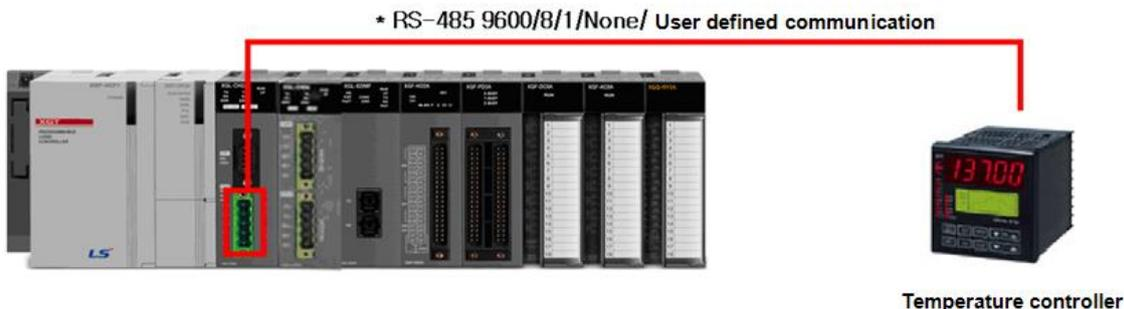
► Connect the PLC and the temperature controller using the Cnet I/F module
