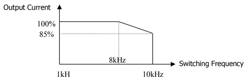
The above graph is only applied when the inverter is operated in the allowable temperature.
