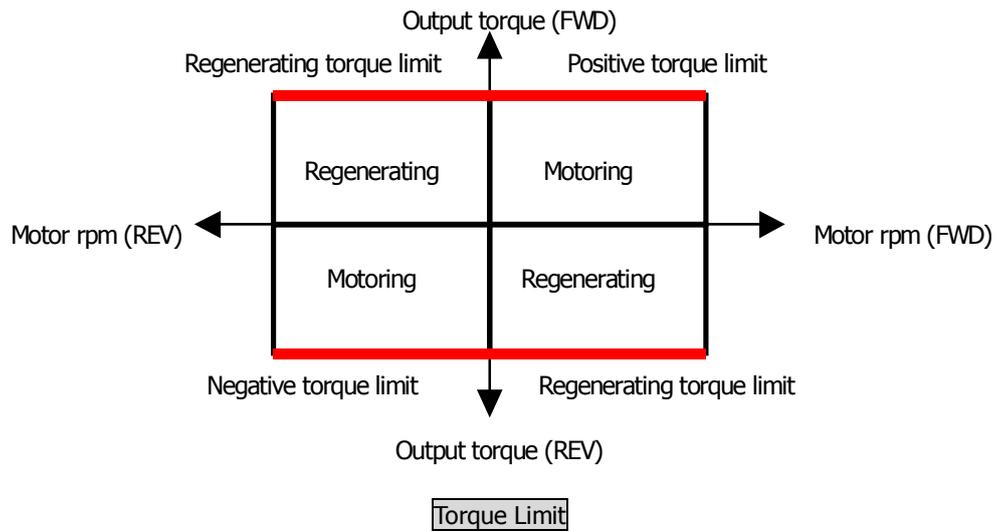
Torque Limit value is determined one of the 9 different combinations shown below depending on CON\_28 setting.
