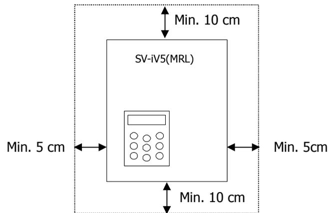
2.1.7 Special care should be taken in case the inverter is to be installed in the panel.
