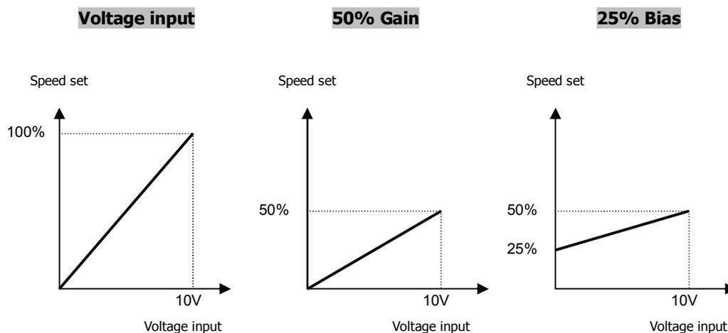
Maximum of the setting value depends on the Gain and starting point on the Bias. In the example above, Maximum value is set to 50% by the Gain and starting point to 25% by the Bias. Consequently, 25 to 50% of the analog command value is effective for 0 to 10V of input voltage.
