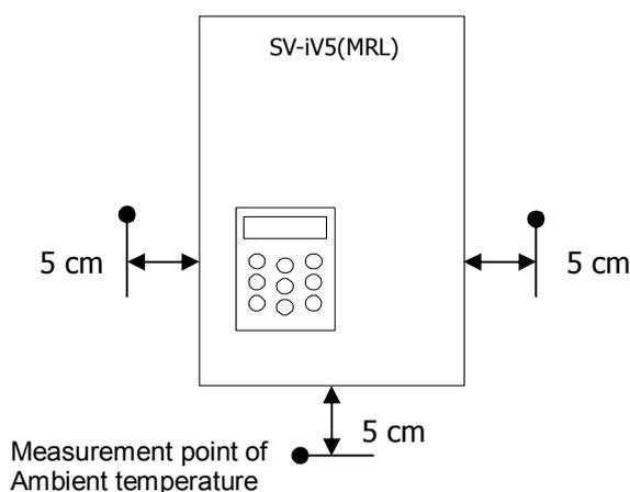
2.1.3 Install the inverter on the unflammmable material. The inverter operates at high-temperature.
