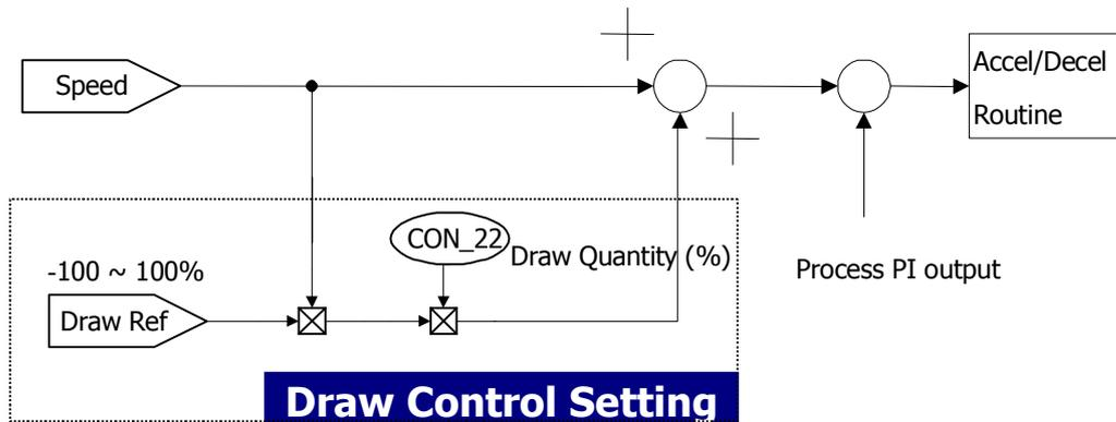
One of the multi-function analog input is set to the draw command ranging from -100% to 100% and the speed command multiplied by Draw quantity is added up to the speed command (Speed Ref) to obtain the final speed command.
