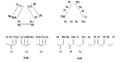
NOTE: 1) Connect lead L1-L7-L7 to line. 1) To reverse rotation interchange any two line lead.
